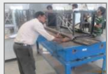
Hoist Mast Inspection on Surface Table for Twist & Bend
